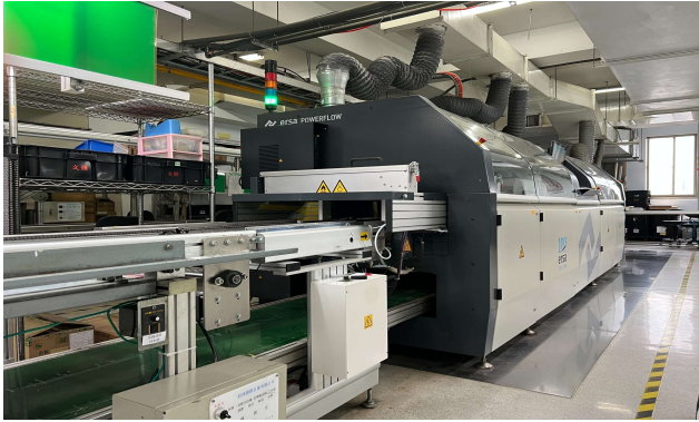
Manual Insertion Line +Ersa Wave Soldering
