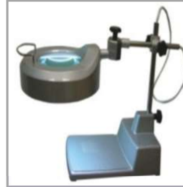
Visual inspection Magnifier
